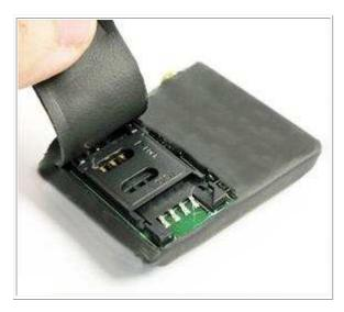
The Digital GSM Spot Wiretap **SIS-WT-2810-Li** is a miniaturized GSM transmitter equipped with voice and vibration detector.
